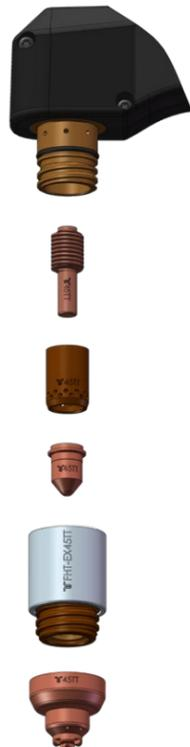
The high-performant FHT-EX®45TT H/M hand and machine torches are ideal for meeting tough demands in continuous operation. These torches are optimally designed for use with EX-TRAFIRE®45SD power supplies and are suitable for cutting, gouging and grid-cutting. They can cut plate thickness of up to 25 mm and more precisely and quickly.
